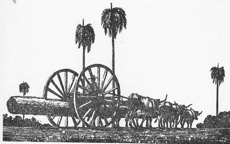
Fig. 1. An alsa-prima used in Alto Paraguay for extracting logs from the forest.
